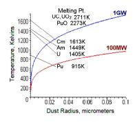
Figure 5. Equilibrium fuel particle temperature as a function of particle size.
