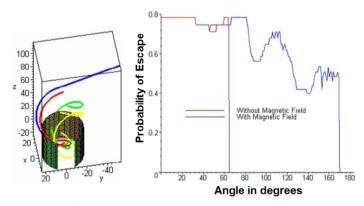
Figure 4. a) Trajectories of fission fragments from dust cloud, which reflect and exit the system. b) Histogram of escape probability for fission fragments as a function of direction and magnetic field.
