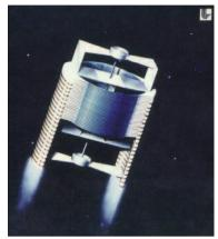
Figure 1. Fission fragment concept as proposed by Dr. George Chapline. The reactor consists of thin carbon filaments coated with nuclear fuel rotated at high speed through the core. Courtesy of LLNL.
