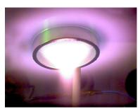
Figure 7. Magnetic quadrupole confinement of ion plasma.
