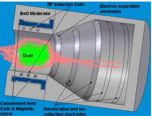
Figure 2. Schematic of proposed Fission Fragment Rocket. Fissile dusty plasma fuel is confined to dust chamber, where RF induction coils heat the plasma. Fission fragments are collimated by the magnetic field either to collection electrodes for power, or exit the reactor for thrust.
