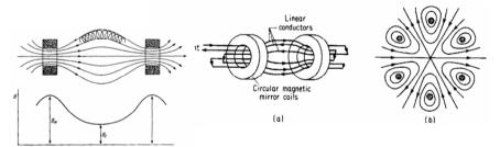
Several magnetic field configurations are possible, the simplest being a magnetic mirror concept as shown in figure 6a. The field strength requirement for a simple coil can be reduced, however, by supplementing with multiple current loops around the perimeter such as the hexapole shown in figure 6b, which can reduce the individual coil strength re-
